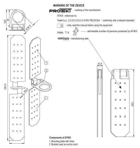
**TIME OF USAGE** - The anchor point can be used for 5 years from the date of the first use. Following the first five years of usage the manufacturer's inspection must be carried out.
