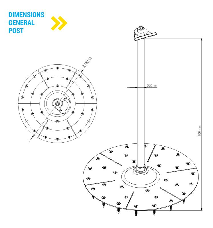
The HLP 700 universal safety post is an anchoring device in accordance with EN795: 2012 type A and CEN / TS / 16415: 2013. The safety post is made of stainless steel for 3 users working simultaneously, with a static strength of min. 14 kN. The post is designed to be fixed to OSB boards with a minimum thickness of 12 mm with screws JT3-ST-2-6,0 x 35. HL 700 complies with the Regulation of the European Parliament and of the Council (EU) of March 9, 2016 on protection measures 2016/425.
